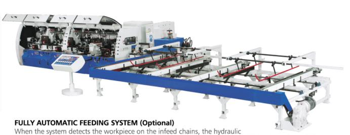
feed system will pneumatically lower and activate the top roller to feed the workpiece into the machine.
